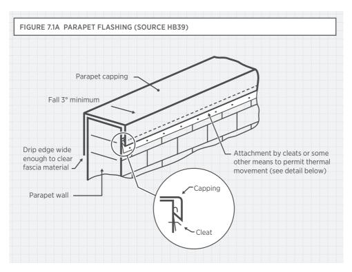
Extract from AS Handbook HB39 - 2015 - Installation Code for Metal Roofing and Wall Cladding<sup>6</sup> <sup>6</sup> Reproduced with permission from SAI Global Ltd under licence 1902-c082.
